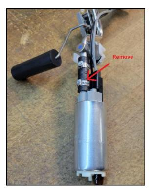
3. Remove the electrical connector to the pump. The connector has a lock that needs to be depressed while removing the connector. This is most easily done with a small flat blade screwdriver.
