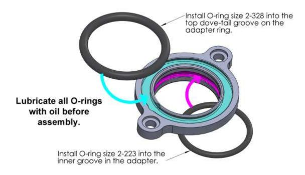
Assemble the thermostat and adapter to the engine.
