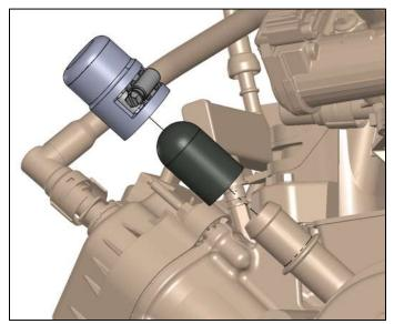
**300-901 heater line adapters (not included) -** Before installation, remove the original top heater tube from the top front of the engine block. Oil all O-rings and mating surfaces before assembly.
