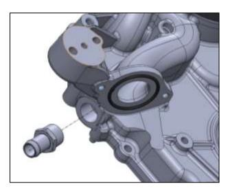
If using the Holley timing cover and accessory drive, install the NPT adapter as shown to left. If using the original timing cover, use the factory installed upward pointing nipple.
