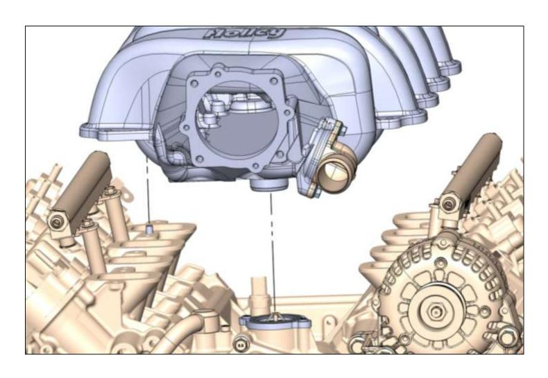
Install the 10 - M6 X 20 Flange Head Bolts to the intake. Hand tighten, then torque in the sequence below.
