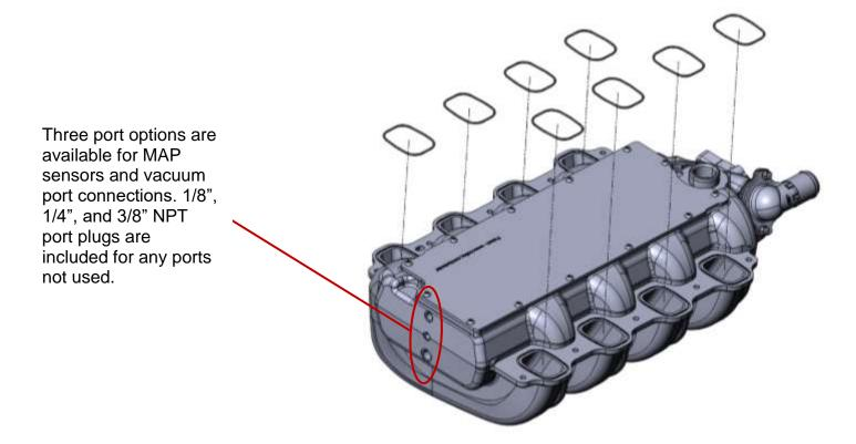
**NOTE:** On all NPT adapters, use thread sealant (Loctite® brand 567 pipe thread sealant or equivalent). Install to finger tight, and then tighten 2 to 3 full turns.
