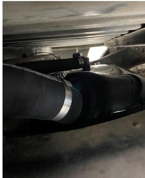
**Figure 1 – Fuel Tank Electrical/Fuel Connections**
