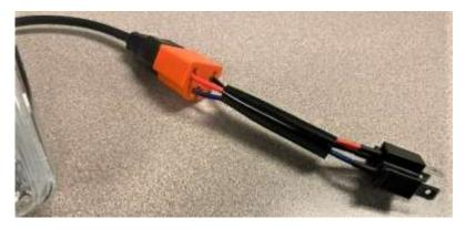
Example shown of what a completed harness may look like. <u>Not all vehicles will match this picture exactly</u>. <u>It is</u> imperative that the vehicle harness is checked to ensure wires are matched properly before powering on.
