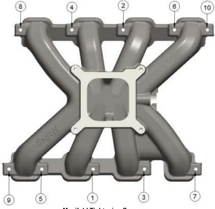
Manifold Tightening Sequence
