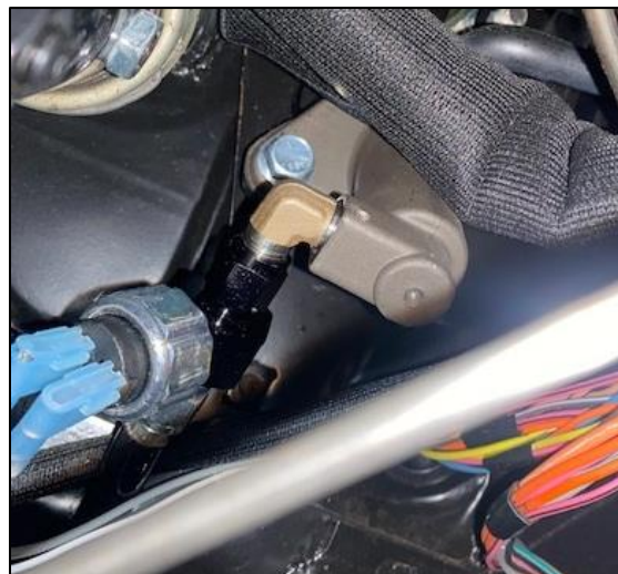
Figure 9: Neutral Safety Switch
