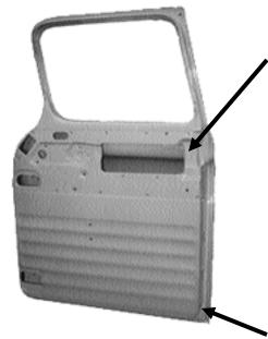
Access hole in door, used when marking the glass on the window sash.
