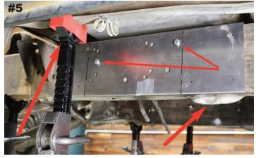
Note mounting location of template is almost butted up to the rear cab mount. Also note location of jack stand under the outrigger and the template notch cut out to clear the spoon like variance found on some frames.
