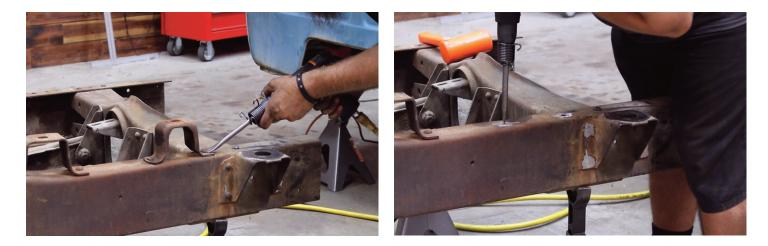
Now that BOTH sides have been drilled, cut-off and the bed and cab mounts have been removed, it's time to relocate the cab mounts. You'll be using the center section of the template that was set aside earlier, but first the Template needs to be prepped.
