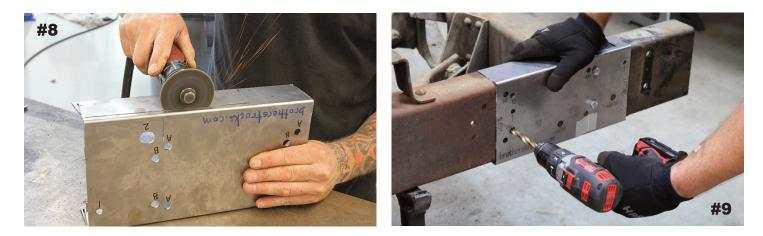
\* With the Template in place, using a 1/8" drill bit, drill the NON-underlined holes that correspond with your year range (72 for '67-'72, 66 for '63-'66) as shown above in #9 on a 67-72 frame.
