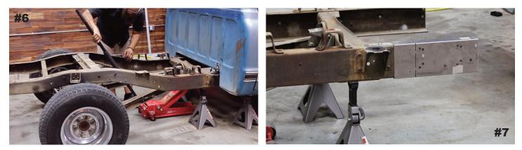
**Template Step 4**. Drill all holes in the panel marked **4 DRILL** on the template using a 1/8" drill bit. Do this for BOTH the DR and PA sides before moving on to Step 5. There are 2 holes on the face of this panel, and 1 additional hole on the top and bottom (total of four 1/8" holes per side).
