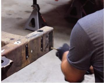
Next, you'll be removing the rear cab mounts and forward most bed mounts from the frame. Using an air chisel (or alternatively a grinder), cut off the heads of the rivets holding the rear cab mounts and forward bed mounts to the frame. Once you have removed the heads of the rivets, use a punch to drive the rivets out of the mounts and the frame (as shown below).
