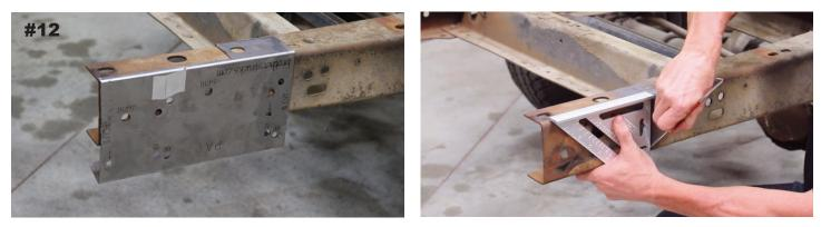
Another part of this step is fabricating an oval hole where your scribe marks are. We have routinely drilled a pair of 1/2" holes side by side and connected them using a grinder, dremmel or boring tool. As an option, you can make a single 1/2" hole aligned on center in the location of the oval scribe marks. This hole is your rear bed mounting hole and may need some amount of front to rear adjustment if you choose to make a single hole. Repeat on BOTH the DR and PA sides.
