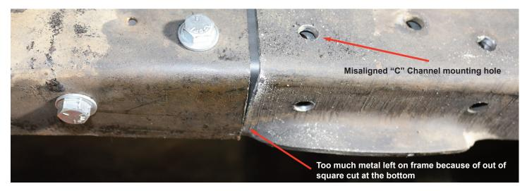
Using the supplied 3/8" hardware, attach the "C" Channel to the rear half of the frame. The channel will align to the forward holes left by the removal of the cab mount, and the 3/8" holes you drilled during Step #4.
