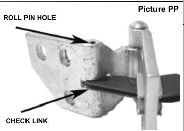
(24) The door check link interferes with the front glass run channel and must be modified. The check link hits the front run channel when closing the door and causes the window bind and not completely roll up. The check link needs to be removed and modified. To remove the check link, you must knock out the check link retainer roll pin on the hinge and pull it out through the door (**Picture PP**). You may choose to take the hinge completely off the door and cab to make modification easier.
