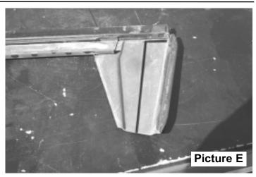
(6) With the glass off the sash. Mark the sash (**Picture E**) and cut with a hacksaw or other cutting tool. The cut doesn't have to be perfect you just want enough room on both sides for the bolts to go through the bracket in the next step.
