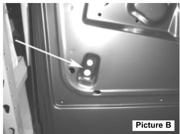
The above picture shows the two bolt holes at the bottom, front of the door where the bottom of the vent window assembly attaches to the door.
