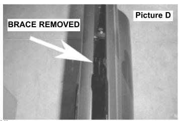
(4) Using a hacksaw or other cutting device, cut the vent window support from the door (**Picture C**). Cut flush with each side of the door (**Picture D**).
