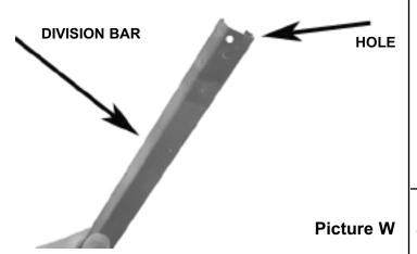
(15) At the top end of the division bar there is a small hole approximately 1/8" from the end (**Picture W**). This hole will be at the bottom of the front glass guide channel. Measuring from that end up, cut the division bar with a hacksaw or other cutting device to 27-1/2" long. This is your front guide channel. Now set it to the side we will come back to it later.
