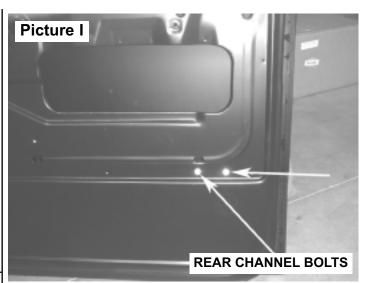
Above picture of lower rear channel bolt holes.
