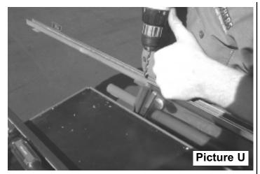
**(14)** Disassemble the vent window assembly by drilling or grinding out the rivets (**Picture U**). Separate the division bar from the rest of the components, it will become the front glass guide channel (**Picture V**).
