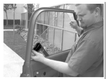
(3) After you remove the vent window assembly proceed to remove the window glass. This can be done by rolling up the glass approximately 3" from being all the way down, then remove the rear roller from the track. Proceed to slide the window back to allow the front roller to be removed from the track. Now carefully lift the glass up from the rear and remove from the door.
