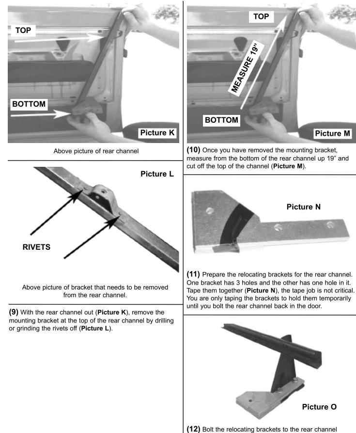
(12) Boit the relocating brackets to the rear channel (Picture O, Picture P, Picture Q) using the  $\#1/4 \ge 20 \ge 1/2$ " panhead phillips screws provided (Picture R). Pictures continued on the next page.
