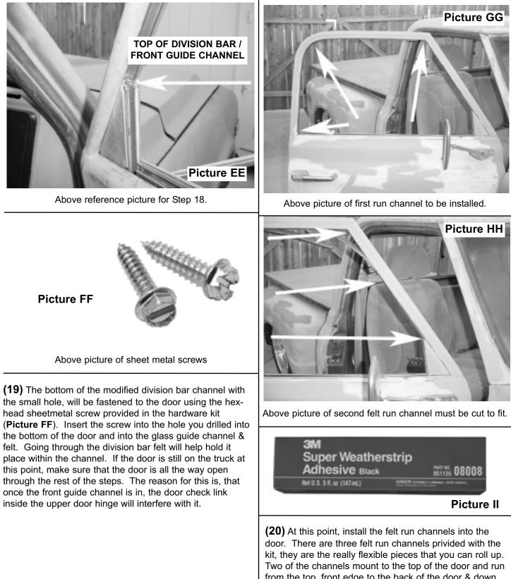
Two of the channels mount to the top of the door and run from the top, front edge to the back of the door & down into the door like your original (**Picture GG**). The third piece will need to be cut into two pieces & will fit into the door from the top of the corner wedge to the top edge of the vent window brace (**Picture HH**). To keep the the weatherstripping from moving in the channel, use **BROTHERS** 3M weatherstripping adhesive, part # is PER8008 (**Picture II**).
