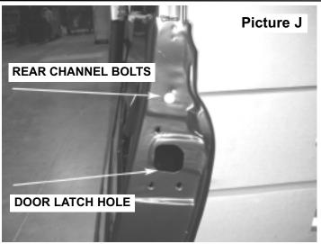
Above picture of top rear channel bolt on the back of the door
