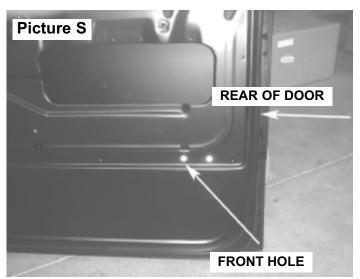
Above picture of the bolt hole used to attach the rear channel with the new bracket.
