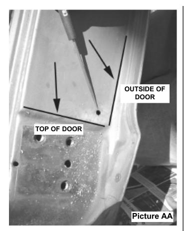
Use the black lines in the (**Picture AA**) for reference on where to measure from to drill the hole.
