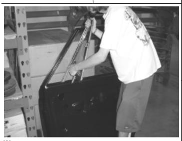
(2) Remove the complete vent window assembly by unscrewing it from the door. There are be three screws at the top, front edge of the vent window (**Picture A**) & two retaining bolts at the front, bottom of the door (**Picture B**). May require some manipulating in order to remove the vent window assembly, it is a tight fit.
