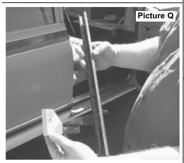
Above picture of rear channel with brackets attached.
