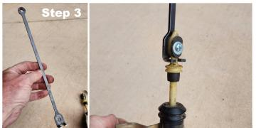
Attach the popper rod extension using the hardware supplied with your power door lock supplement.
