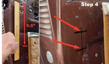
Mark a new pair of holes exactly 9.5" below the original holes and drill them out with a 5/16" drill bit.
