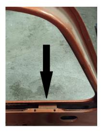
Take the glass run channel provided in the kit and place it DRY (without glue or adhesive) into the door. Take your time and reshape the channel to your door. Once the main shape is made, glue only the top of the channel into place. You will need to take the inner door molding off. This will allow you to see the channel when installed.
