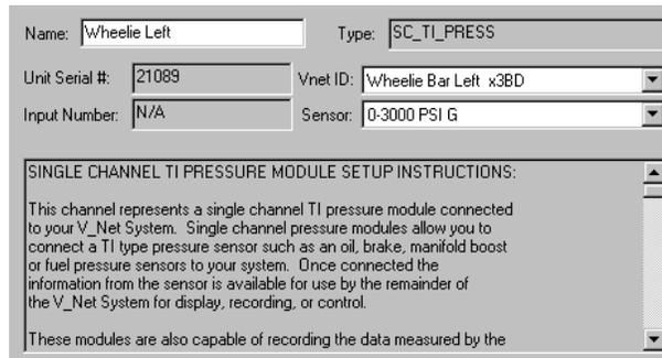
Locate the text box labeled **Single Channel TI Pressure Module Setup Instructions**. This text box provides online instructions for modifying the setup of this module. Read the instructions and modify the setup as desired. (Please note the scroll bars located on the left- hand portion of the text box are used to scroll through the instructions).
