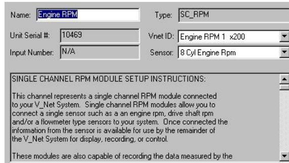
Locate the text box labeled **Single Channel RPM Module Setup Instructions**. This text box provides online instructions for modifying the setup of this module. Read the instructions and modify the setup as desired. (Please note the scroll bars located on the left- hand portion of the text box are used to scroll through the instructions.
