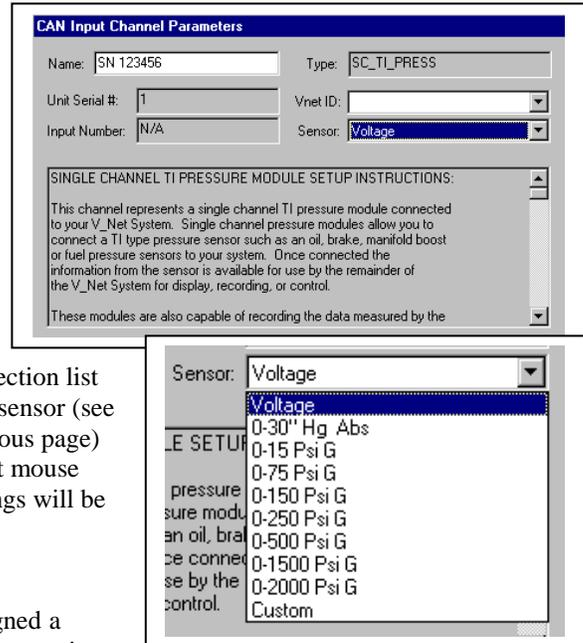
When you have finished editing the configuration on your PC, you will need to send the information to the sensor module. Be sure the serial interface cable is connected to your V50 unit or data logger and power is applied to the system. To send the information position the mouse cursor over the **Send Configuration** button and click the left mouse button. The progress box as shown to the left will be displayed.
