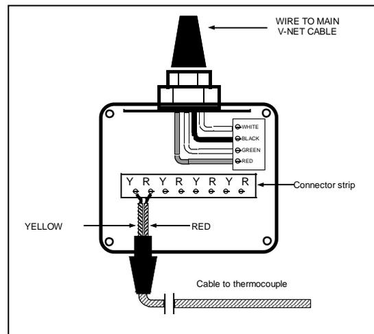
The next step is to insert the V\_Net cable tee wired to the module into the V\_Net data bus in your vehicle. The V\_Net cable tee can be inserted at any location in the V\_Net cable in your vehicle. Select a location where the connector module can be mounted safely. Avoid mounting near heat sources and high voltage ignition wires.
