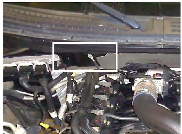
11. Find a suitable location on the passenger-side of the firewall to mount the dipstick adapter (3), while also looking for a suitable route for the dipstick tube.
