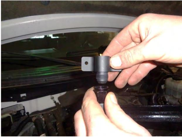
17. Thread the adapter to the top of the tube, but leave the nut loose at this time.
