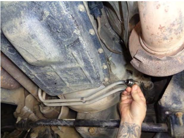
8. Temporarily re-install the stock fill cap, then turn off the vehicle. **NOTE: If the cap is not installed when the vehicle is turned off, the hot (expanded) transmission fluid may overflow the fill port as it returns to the pan.**
