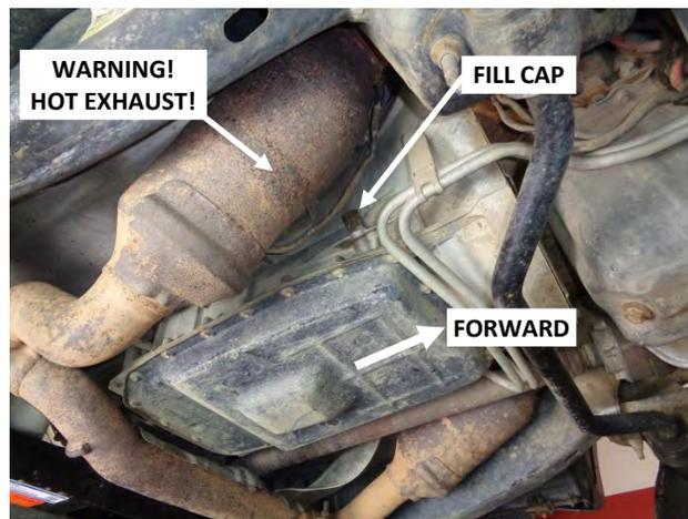
4. Under the vehicle, locate and remove the transmission fill cap. (It is located on the passenger side of the transmission, above and toward the front of the pan.) **WARNING: The exhaust system is extremely hot. Wear suitable gloves and long sleeves to avoid burns.**
