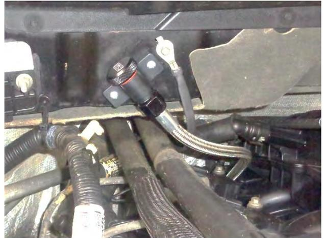
20. Wipe the dipstick and wire with a clean, lint-free rag to remove any rust preventative oil. Then install the dipstick in the tube, and tighten the knob fully hand-tight (until the o-ring is compressed).
