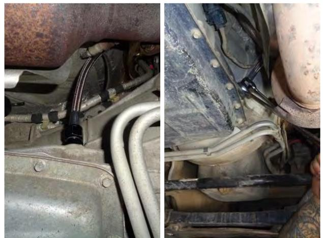
16. Assemble the dipstick tube to the fitting and tighten the nut. **Turn off the vehicle if it is running.**
