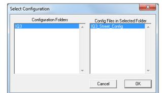
7. The list on the right will now contain the list of configuration files contained in this folder. Select the appropriate Racepak device you intend to communicate with and click the OK button.
