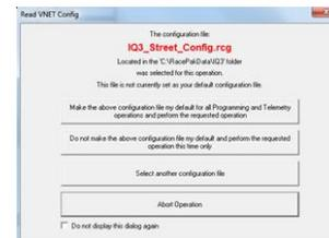
11. A dialog box (shown right) may appear asking if you wish to make this configuration the default configuration file. If this is the only Racepak system you will be programming, select the top option to make it the default. If using this PC to program more than one Racepak system, select the second box.
