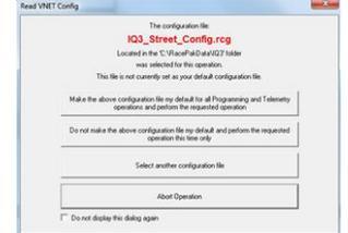
10. A dialog box (shown right) may appear asking if you wish to make this configuration the default configuration file. If this is the only Racepak system you will be programming, select the top option to make it the default. If using this PC to program more than one Racepak system, select the second box.
