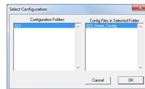
7. The list on the right will now contain the list of configuration files contained in this folder. The factory configuration file for the IQ3 Street Dash unit will be located here.
