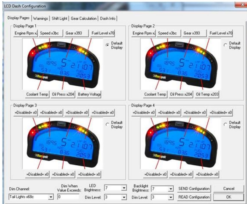
A view representing the current programming of all four display pages is obtained by selecting the Display Pages tab. Each input is programmed by selected the text box related to that input area, as indicated by the red line extending down to the dash, from each text box.
