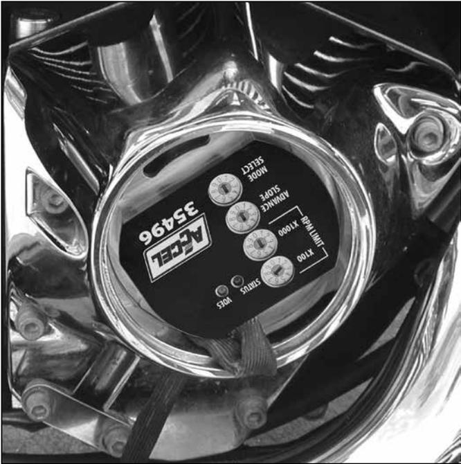
Figure 2 - Installing Unit (Note Orientation)
