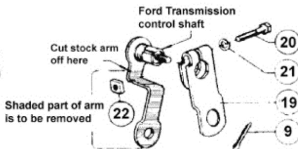
Cut shaded part of stock arm off. Install Hurst arm on shaft loosely using the supplied hardware. Do not tighten at this time. Follow the adjustment procedure outlined in the body of the instruction sheet.
