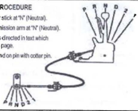
With shifter mounted in the desired location, direct eyelet end of shifter cable through shifter frame. Secure shifter cable to frame using cable clip (#4), push clip down until it is firmly seated. Put shifter in neutral and slide cable eyelet over pin on shifter stick (see exploded view), install cotter pin (#3) through hole in shifter pin to hold cable in place.
