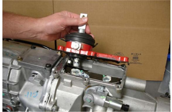
Install the rubber boot onto the Blackjack shifter. Confirm that the rubber boot does not interfere with shifter movement and that the shifter lever movement is not restricted or binding at full travel positions. Failing to do so could result in the shifter popping out of gear and damaging the transmission.
