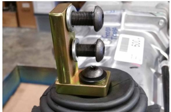
Attach the Chrome Hurst shift handle to the lower stub stick using the supplied hardware. Reinstall the shift boot and factory console. If you are using a properly designed crossmember and your car is in good condition (no floor sag, stock height sub-frame mounts that are not worn, and properly aligned sub-frame), there will be no modifications required to your floorboard or console when using this shifter.
