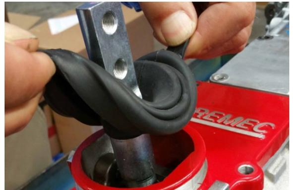
The shifter "body" will be in the in the forward position on the rear T56 shifter cavity. Make sure the pivot ball is positioned into the rear socket and that the white plastic bushing is still in place.
