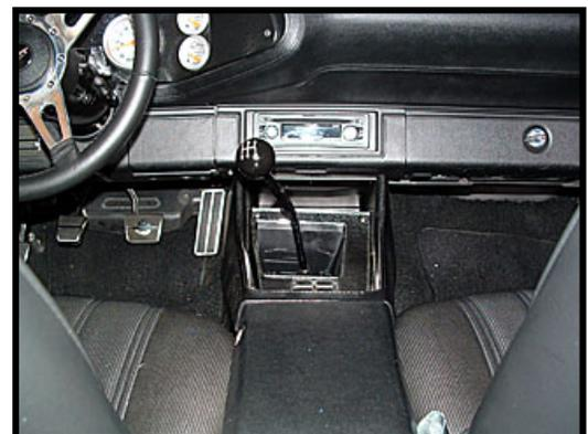
Install the shift knob onto the stick. Align the logo on the shift knob accordingly and tighten the jam nut up against the knob. A few drops of Loctite will help prevent the knob from loosening.
