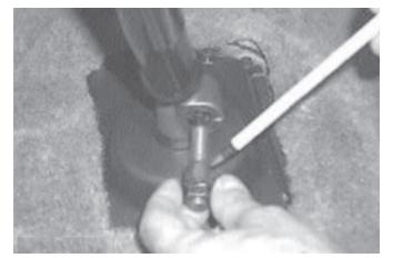
5. Remove shifter stick from shifter mechanism by removing hex flanged nut then installing it on opposite side. Tighten nut to draw out stud, then pull shifter stick up and off.
