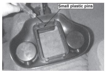
24. To re-install factory console, remove factory boot by snapping off small plastic pins securing boot to under-side of console.
