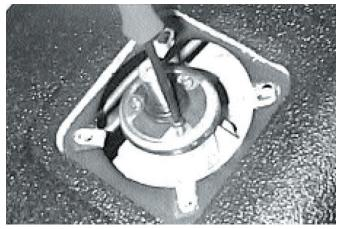
Remove (x3) screws securing shifter base to transmission and remove shifter mechanism by pulling up and out.
