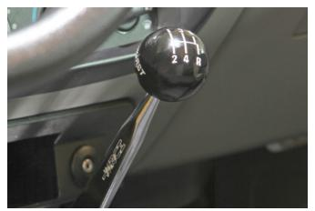
34. Install shifter knob onto shifter stick.
