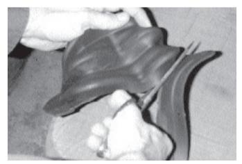
25. Carefully cut flange (directly below bottom fold) off of Hurst Superboot.
