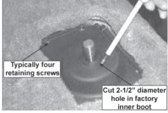
6. Remove factory inner boot and plate assembly from floor tunnel by removing (x4) screws.
