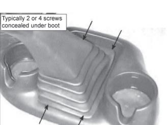
3. Remove screws securing console and shift boot to floor tunnel.
