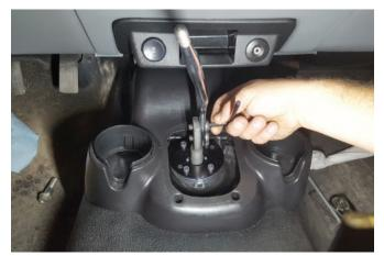
**32.** First, re-install console, then shifter as shown.
