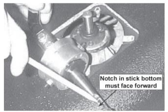
13. Position Hurst shifter assembly onto mounting plate with notch in stick bottom facing forward.
