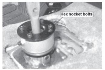
**NOTE:** If your vehicle required a spacer (step 12) use (x4) longer bolts now in place of bolts removed step 8.
