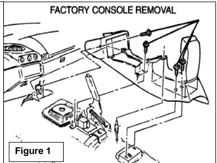
6. Raise the console at the rear and disconnect the electrical wire socket located on the console. Pull the console towards the rear of the vehicle to release the front mounting tabs. Lay the console on its side and remove the ash tray light socket.
