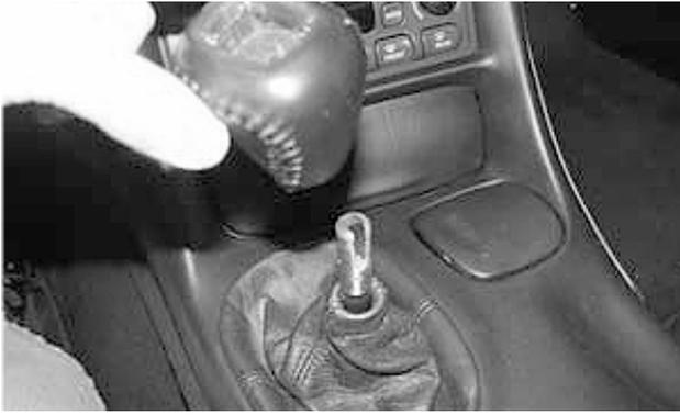
29. Thread the shift knob onto the shift lever, aligning the keyhole with the keyway in the shift lever.
