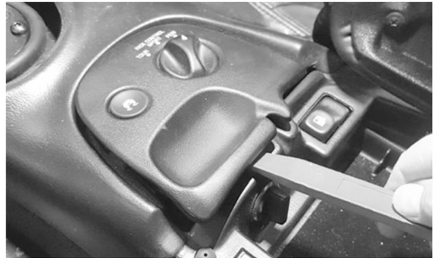
8. **At the front edge of the storage compartment,** lift up on the rear edge of the half-round panel to detach it from the front console. Disconnect any electrical plugs, and set the panel aside.
