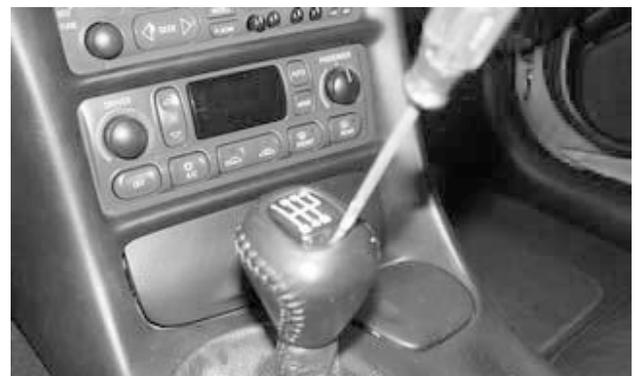
2. Remove the shift-pattern insert from shift knob with a small, flat-tipped screwdriver.
