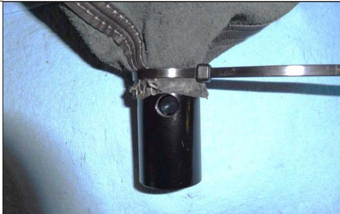
43. Reinstall the factory isolation boot onto the Hurst pistol grip as shown.
