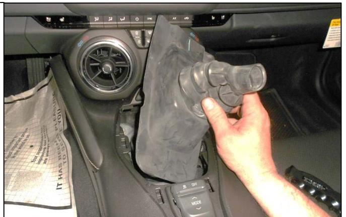
6. Using an extension and 10mm socket, remove the 4 bolts attaching the rubber boot to the transmission tunnel.
