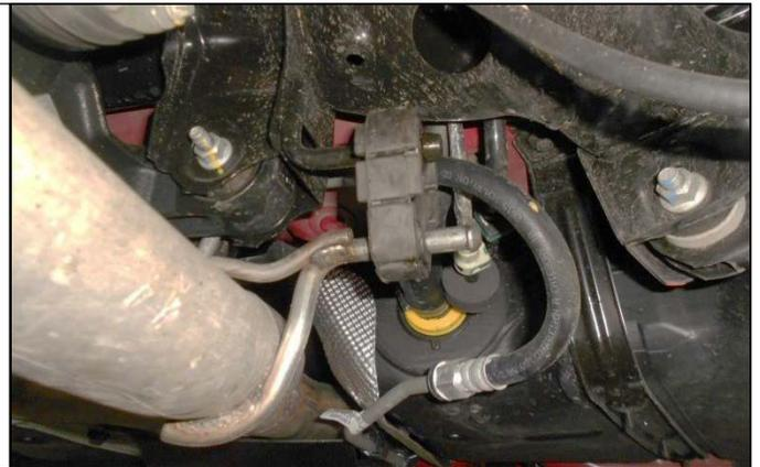
12. At the rear of the vehicle there are two mounted hangers located on the left and right side. Remove the two 15mm nuts that attach each hanger then remove the hangers.
