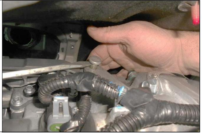
27. Reposition the screw driver between the rubber isolator on the shifter housing and push the spring lock in and remove the pin.
