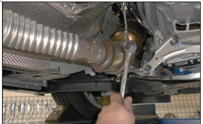
10. Loosen the 15mm nut from the right side exhaust flange connected to the catalytic converter. Spread the clamp open.
