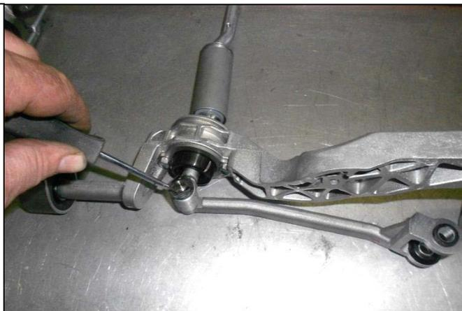
31. Remove the factory shifter from the housing by unbolting the two 10mm bolts and removing the mounting ring.
