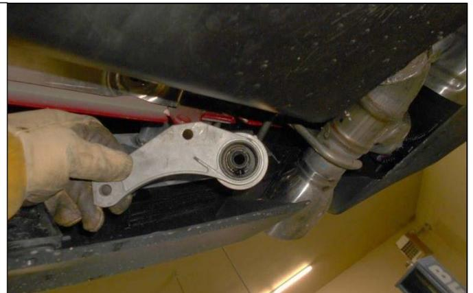
13. The right front exhaust flange is a ball socket you can pry between the transmission cross member and the exhaust to pop it out.
