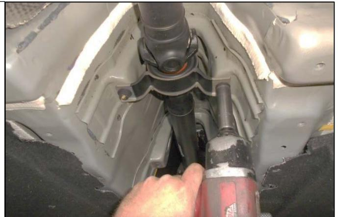
21. The drive shaft can be squeezed together in order to clear the transmission and differential flange.
