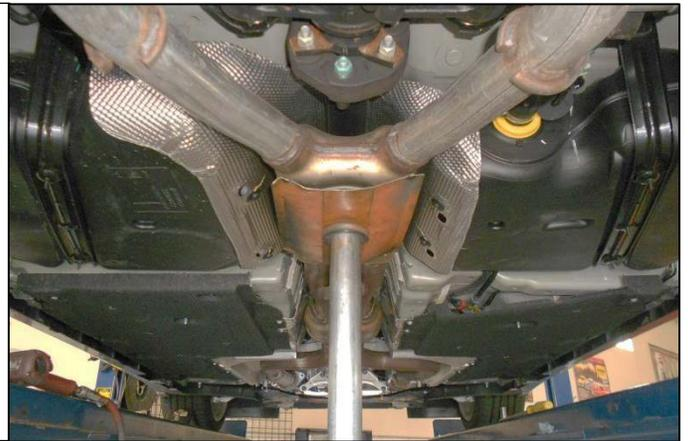
9. Remove the two 15mm nuts attaching the left side exhaust flange to the catalytic converter.
