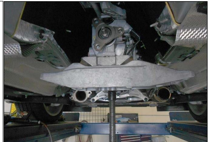
25. The shifter housing is connected to the transmission with a pin on the left and right side. The pin has a spring lock at the end of it as shown here.
