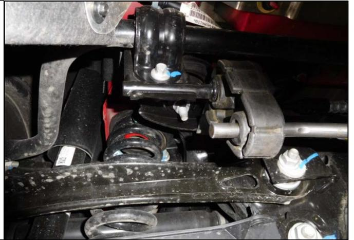
15. Remove the four 13mm bolts from the tunnel brace and remove the brace.
