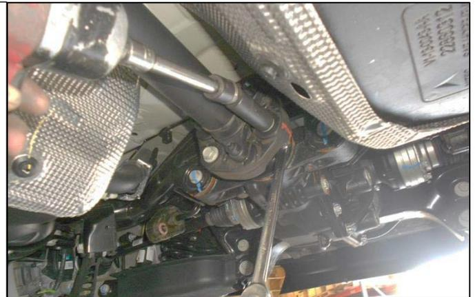
20. Support the drive shaft. Remove the two 15mm bolts from the center carrier bearing. This will allow the drive shaft to be removed from the vehicle.
