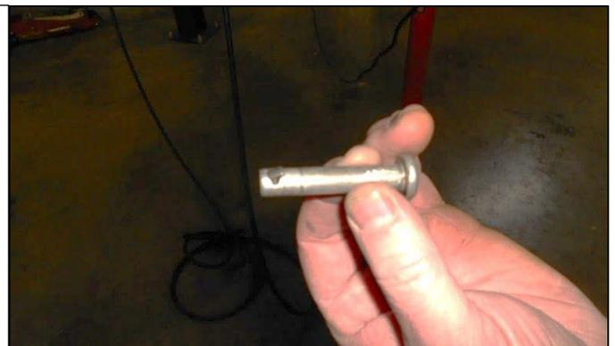
26. Remove the pin on the left and right side by pushing the spring lock down while using a screw driver to pull the pin out until it stops.
