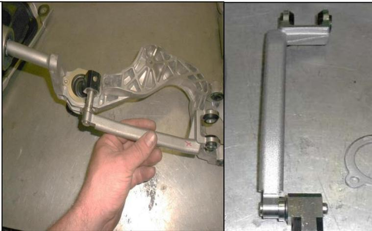
35. Verify that the factory shift rod is oriented in the same position as when it was removed.
