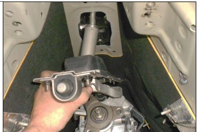
30. Remove the spring clip from the factory shift rod and remove the rod. Take note of the shift rod orientation.
