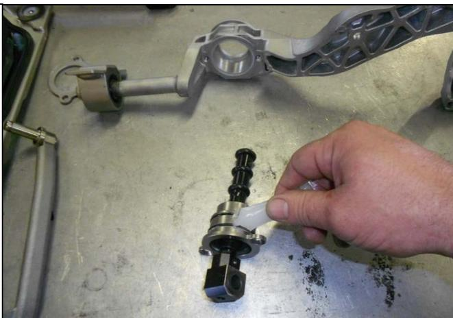
33. Install the Hurst shifter assembly in into the factory shifter housing. Bolt this in place using the provided M6x10mm counter sink bolts.
