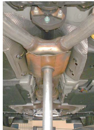
9. Support exhaust then remove (x2) 15mm nuts attaching left side exhaust flange to catalytic converter.
