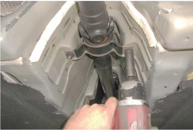
19. Support drive shaft then remove (x2) 15mm bolts from center carrier bearing.
