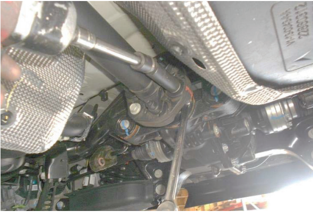
18. Remove (x3) 18mm bolts and nuts from flex coupling and differential flange.
