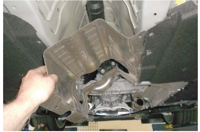
15. Remove (x3) 10mm bolts and heat shield from vehicle.
