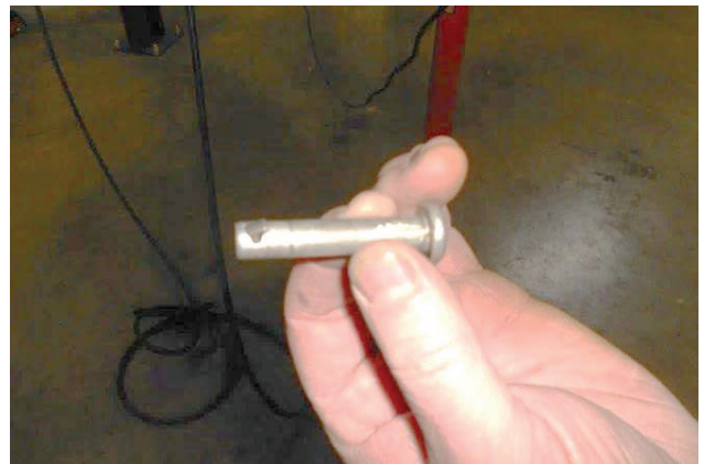
23. Shifter housing is connected to transmission with a pin on left and right side. The pin has a spring lock at its end as shown.
