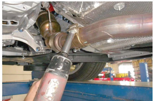
10. Loosen 15mm nut from right side exhaust flange connected to catalytic converter then open clamp.
