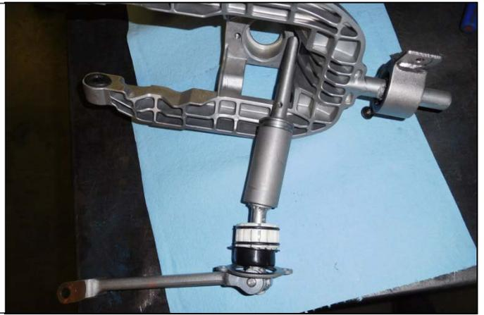
34. Inset all four flange bushings into the supplied link bar. Ensure that the flange portion of the bushing is on the inside of the rod.
