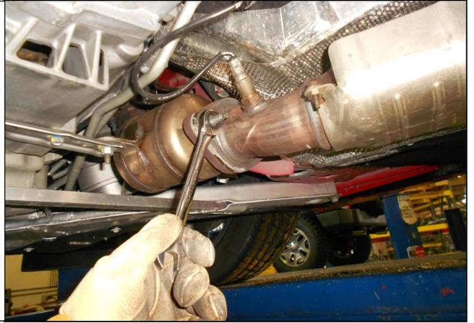
10. Unplug the oxygen sensor that is attached to the right side exhaust. Make sure it is free and clear.
