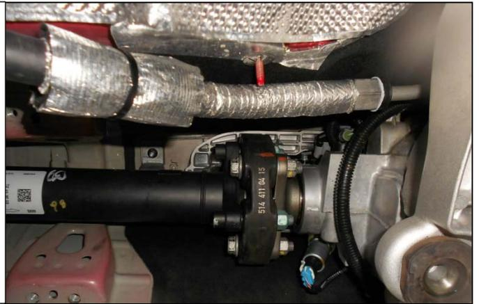
18. Remove the three 18mm bolts and nuts from the flex coupling at the transmission.
