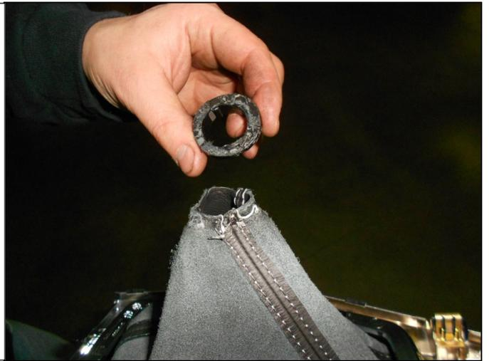
45. With the boot inverted, install the Hurst pistol grip shifter through the boot.
