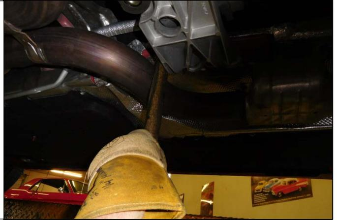
14. Remove the mid hangers on the left and right side of the exhaust. The entire exhaust system can now be removed.
