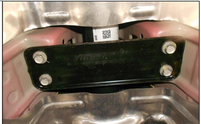
16. Remove the three 10mm bolts from the right and left side of the heat shield. Remove the heat shield.
