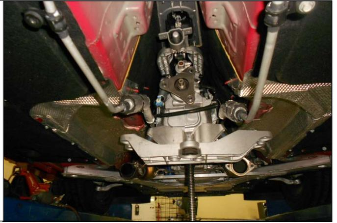
26. The shifter housing is connected to the transmission with a pin on the left and right side. The pin has a spring lock at the end of it as shown here.
