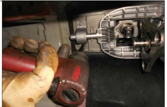
24. Remove the four 15mm bolts from the transmission cross member
