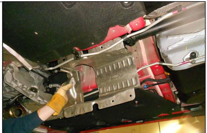
17. The drive shaft must be removed. Start by making an alignment mark on the flex coupling and the transmission flange.
