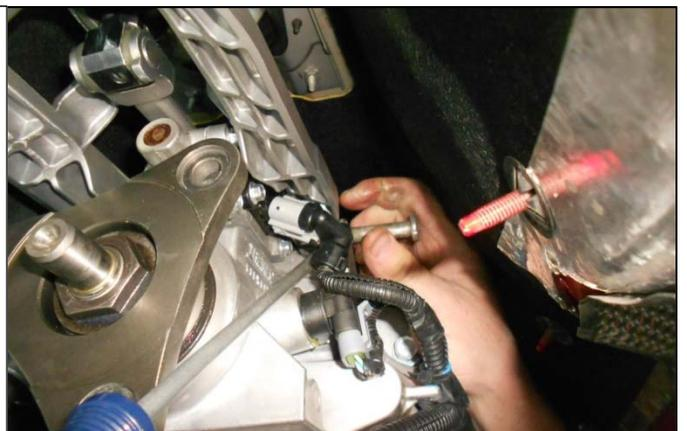
29. Remove the spring loaded clip from the cross pin that attaches the shift rod to the transmission and remove the pin.
