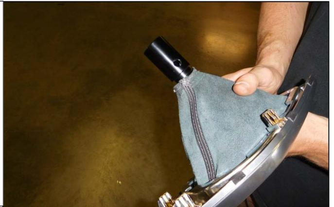
46. Ensure that boot is past the machined groove on the pistol grip and is orientated in the right direction. Secure the shift boot to the pistol grip using the supplied tie wrap.
