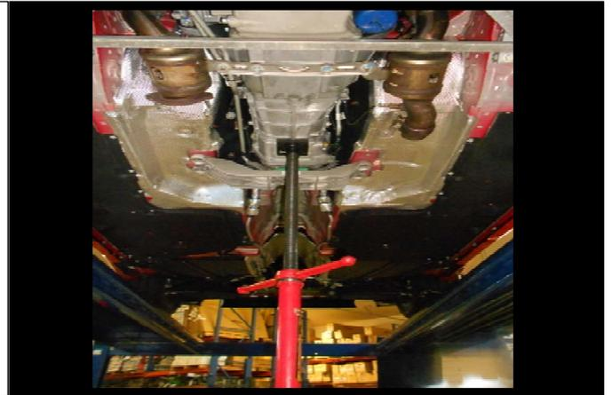
23. Remove the two 10mm bolts from the rear of the shifter housing.
