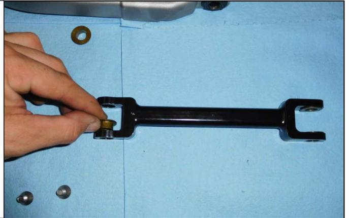
35. The Hurst shifter assembly and the link bar can now be assembled.
