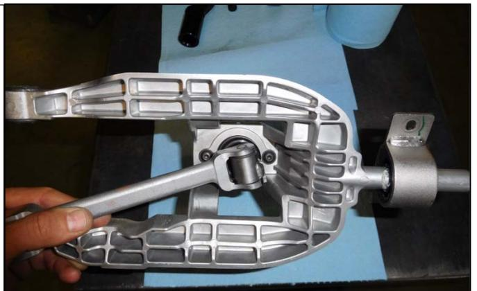
33. Remove the stick assembly from the shifter housing.
