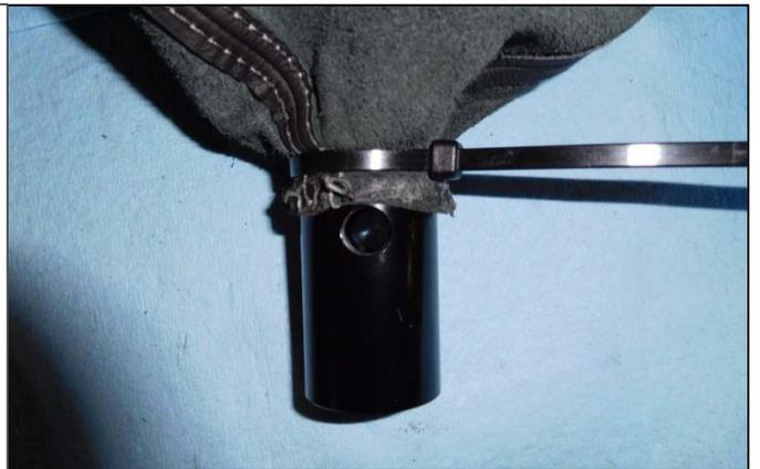
47. Using grease or soap and water, place some lubricant on the O-rings located on the lower stick. With the shift boot still inverted, slide the pistol grip down over the top of the lower stick. Ensure to align the two holes on the pistol grip to the two threaded holes on the lower stick.
