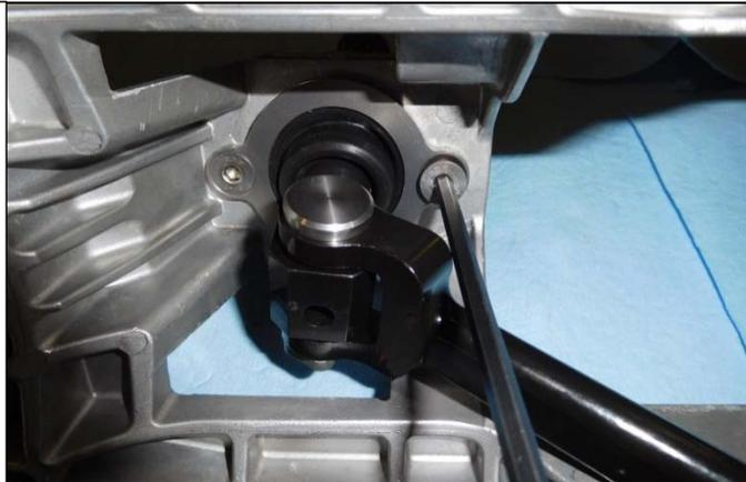
38. Grease the forward bushings on the shift rod and reinstall the factory rubber boot.
