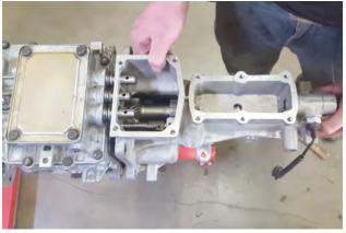
**NOTE:** Apply a small amount of lubricant to (x3) o-rings for shift rails.
