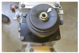
20. Remove boot from factory shifter. Remove bolt and washer from Blackjack shifter then install factory boot as shown.
