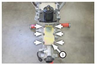
19. Apply rtv or silicone then set **rear cover (3)** onto transmission and secure it with (x6) bolts (removed step 8).
