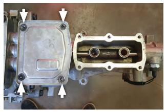
4. Remove (x4) bolts and plate from transmission.
