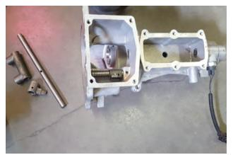
Remove double socket cup then set all parts aside. Make sure to remove roll pin (removed step 10) from the inside of tail shaft housing.
