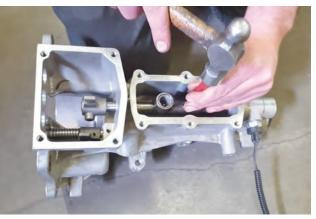
10. Remove roll pin. Make sure it is in neutral then drop roll pin through oil drain hole.
