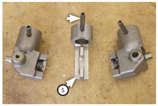
16. Place roll pin (removed step 7) into center lug (5).
