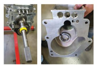
9. Remove tail shaft carefully, making sure not to damage internal components. Then clean faces of both parts to remove any residual adhesive.
