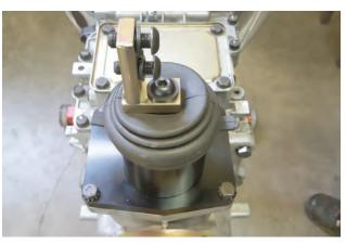
22. Use (x2 ea.) **cap screw (6)** and **split lock washer (4)** to secure shift stick once installed in vehicle.
