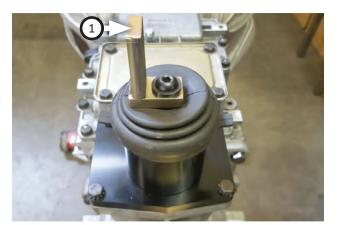
21. Install **offset stick weld (1)** and secure it with washer and bolt (removed in previous step).
