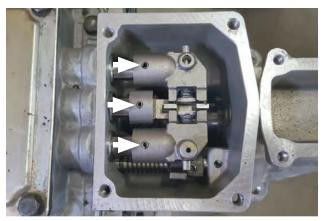
17. Install lugs back onto rails (center first) as shown. Reinstall roll pins to fasten them in place.
