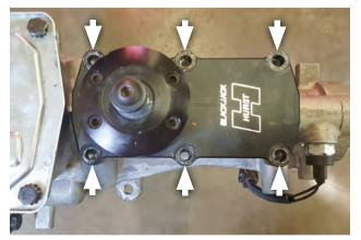
3. Remove (x6) bolts holding shifter assembly in place, then remove it from transmission.
