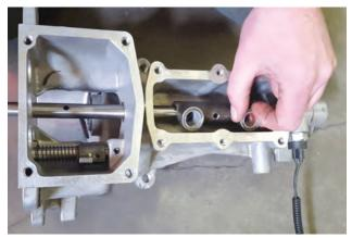
12. Remove lug and shaft from rail, then remove rail.
