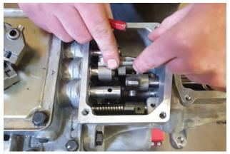
7. Rotate remaining lug to disengage rear shift selector rail, then remove it from shaft.
