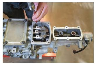
5. Remove (x3) roll pins from forward shift lugs.
