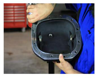
9. Install the B&M differential cover on the axle housing using the 3 OE/stock studs on top right side of cover & the supplied allen bolts and washers. The original stud fasteners are required to accommodate the factory wiring clips/brackets clips/brackets. Torque to factory specs.
