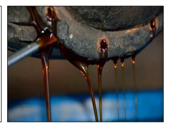
6. Using a dry lint free rag, clean the accessible area of the axle housing and check the internal components for visible excessive wear or other problems.
