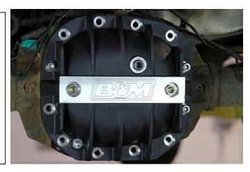
10. Install the supplied magnetic 1/4" NPTF drain plug on the B&M Diff Cover and tighten.
