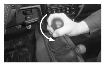
1. Remove the shift knob by unscrewing it from the shift lever.
