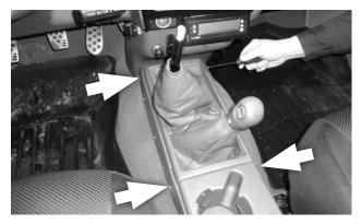
Remove the 2 screws from each side of the front console (4 screws total).
