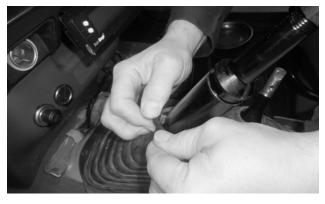
17. Work both boots down the their shift levers. Carefully work the front boot opening past the 2 screw heads, then push it down the lever until it touches the raised lip.
