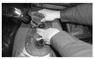
**15. Install the lower dust boot over the shift levers,** and work its front opening down over the rubber boot on the shifter.
