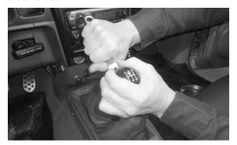
**23. Thread the knob all the way down,** back it off just enough to align it as desired, and tighten the jam nut against it.
