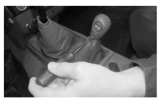
Remove the screw from the side of the transfer case shift knob.
