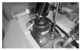
11. Re-install the stock shifter screws, and tighten to 13 ft-lbs.
