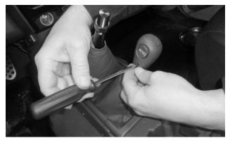
21. Reattach the knob to the transfer case shift lever.
