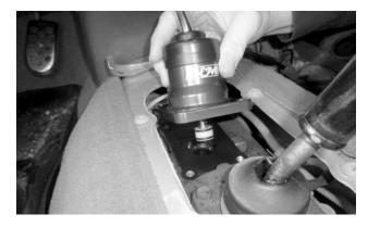
**10. On the B&M shifter, lubricate the pivot bushing o-rings.** Then install the shifter on the mount pad, inserting the pivot bushing into the shift linkage.
