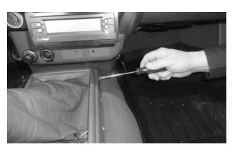
20. Reinstall the 4 console assembly screws, ensuring that the 4WD wire is tucked fully under the console (not caught under the side).
