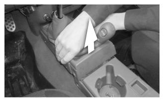
**4. Lift the rear of the front console,** carefully separating it from the center console.
