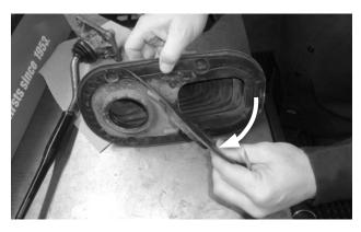
**14. Carefully peel the lower dust boot** off of the cover plate assembly.
