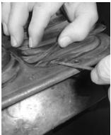
**13.** On the cover plate assembly, remove the four staples that hold the upper and lower dust boots together.
