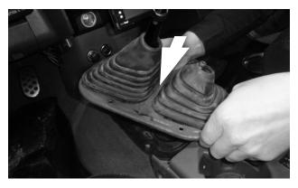
16. Lower the rest of the cover plate assembly over the shift levers.
