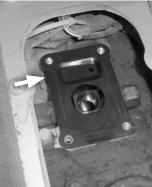
9. If the sheet metal splash plate comes off with the shifter, wipe the shifter mount pad clean, wipe both sides of the splash plate flange, and reinstall the plate back on the mount pad with the tab on the left side pointed down.
