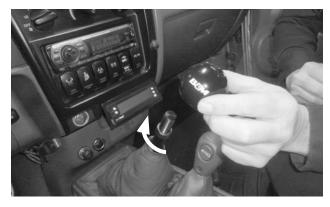
**22. Run the jam nut all the way down the threads,** then install the shift knob.
