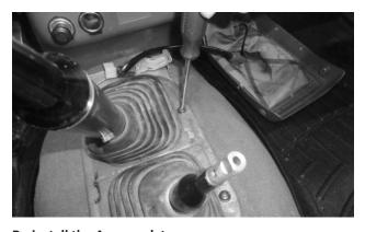
18. Re-install the 4 cover plate screws.
