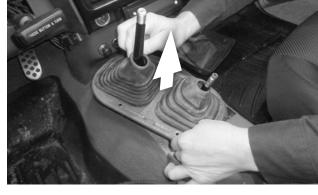
**7.** Work the rubber boots up their shift levers, lift the cover plate assembly over the levers, and set it aside.
