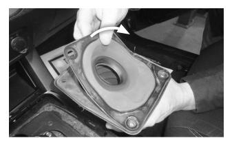
**19. Carefully peel the lower dust boot** off of the cover plate assembly.
