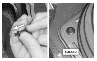
**22. Re-set the plungers on the 2 push-lock fasteners** by pushing them up from the bottom end. Then insert the fasteners in their holes and lock them by pushing the plungers down flush.
