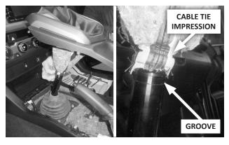
**25.** With the leather boot still turned inside-out, work its opening down over the shift lever until the impression from the old cable tie is located over the groove on the lever.
