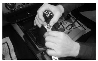
**31. Turn the knob all the way down** until it touches the nut. Then back it off to align it as desired, and tighten the jam nut.
