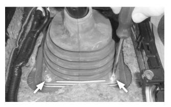
23. Re-install the 2 cover plate screws.
