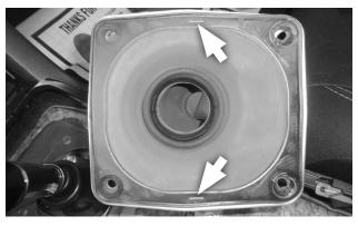
**18. On the cover plate assembly, remove the 2 staples** that hold the upper and lower dust boots together.
