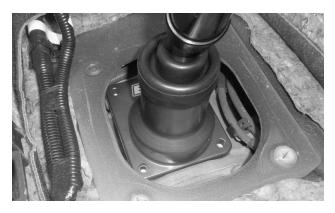
**14. Install the shifter on the mount pad.** First insert the pivot bushing into the shift linkage. Then align the 2 mount pad bushings.
