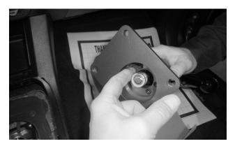
**13.** On the B&M shifter, lubricate the pivot bushing o-rings, and align the bushing with the lever centerline (make sure it's not cocked).
