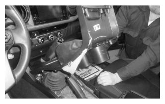
**6.** When the parking brake boot is clear of the lever, remove the console trim panel and set it aside.
