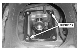
**12.** If either of the 2 alignment bushings, or the gasket, remains with the shifter, return them to their locations on the shifter mount pad.
