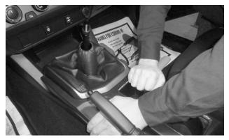
**29. Press the upper console back into place** on the console base. Be sure that all console edges are flush with the base.
