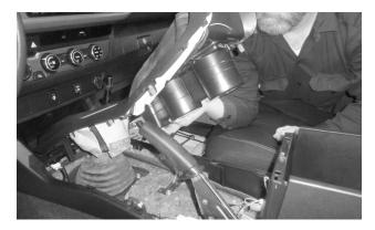
**27. Move the shift lever into THIRD gear** (for clearance), then lower the upper console over the parking brake handle.
