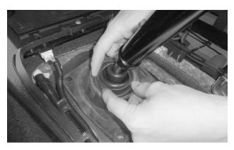
**20. Install the lower dust boot over the shift lever,** and work it down over the rubber boot on the shifter.
