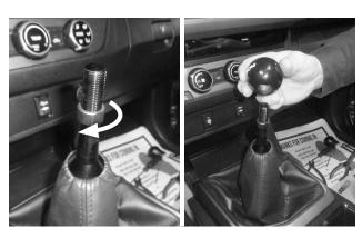
**30.** Run the jam nut all the way down the threads, then install the shift knob.
