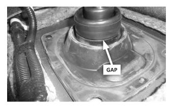
The top edge of the lower dust boot will sit just below the bottom edge of shifter boot. (There will be a slight gap between them.)
