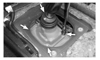
**11. Put the shifter in NEUTRAL.** Remove the 4 mount screws, then remove the stock shifter.
