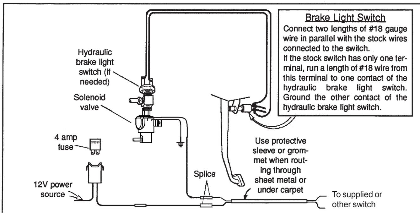
insulated connector. All soldered connections should be wrapped with plastic electrical tape. All wires should be as short and direct as possible, but not short enough to put any tension on the wires. Electrical wires should not be under tension even when the engine and transmission move on their mounts.
