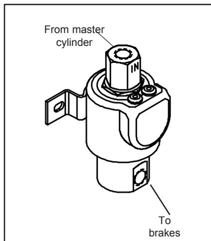
instructions is the same for all systems. Read the instructions thoroughly and identify the additional brake line and fittings that you will require. These lines and fittings are available for most popular vehicles. In order to determine the correct fittings required, a tube nut gauge is included with this kit. The locations to check the fittings are shown on the illustrations for the different types of brake systems.
