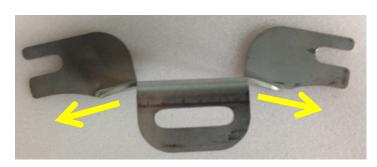
MTBRGMK – After Bending (Bend at thin sections)
