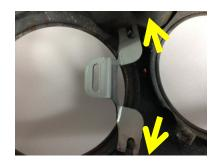
Bent MTBRGMK Installed in Dash
