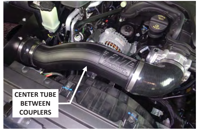
29. Center the intake tube between the couplers, then tighten the 2 remaining clamps.
