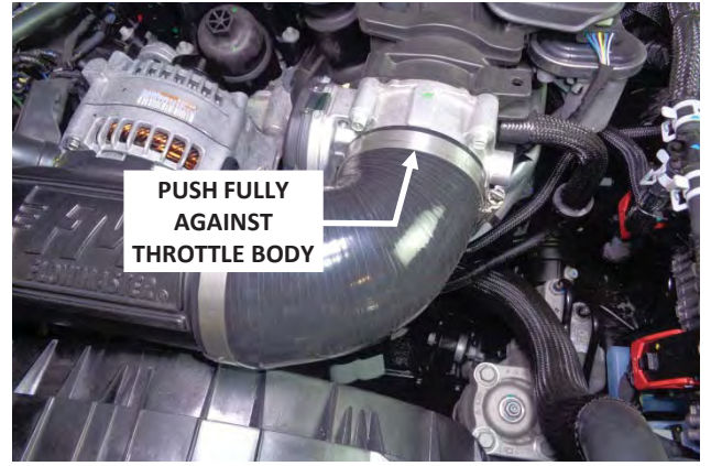
28. Push the elbow coupler up against the throttle body stops, then tighten the throttle body clamp.
