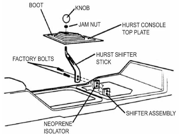
3. Place the console top plate over the shifter and slide the boot down over the stick. Position the top plate onto the console, and carefully push down until the top plate is flush with the console and firmly in place.
