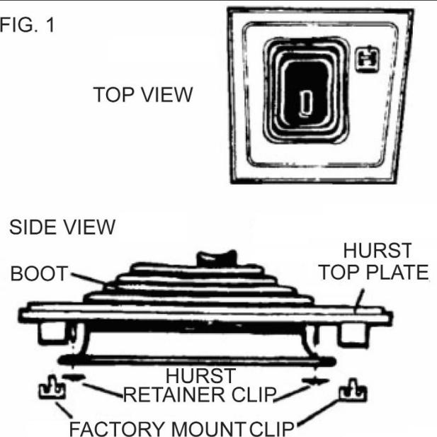
Install the boot with the offset hole to the rear of the top plate
