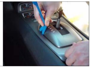
**STEP 6.** Carefully remove the center console trim plate and place it to the side.
