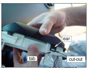
**STEP 20.** Place the Hurst plate and white plastic shifter frame assembly back on top of the shifter. Make sure the white plastic frame clicks onto the shifter, the studs of the center console engage at the screw mounting points, and the ABL LED wires do not interfere with the shift mechanism or black plastic slider through it's full range of motion.
