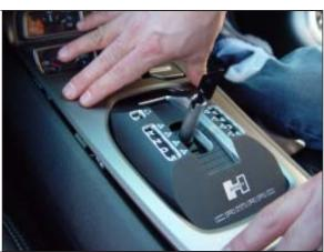
**STEP 24.** Reinstall the shifter knob by sliding it down onto the shifter shaft making sure that the base of the knob properly engages the black plastic slider. Then replace the mounting screw.
