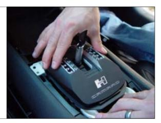
STEP 21. Replace the four (4) mounting screws.
