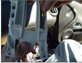
STEP 15. Ensure that the original LED bulb is NOT lit prior to beginning the wiring installation. This may require moving the shift lever to the park position and removing the key from the ignition. In some instances it may be necessary/prudent to disconnect the vehicle battery (refer to the vehicles service/owner's manual) to avoid problems with improper wiring.
