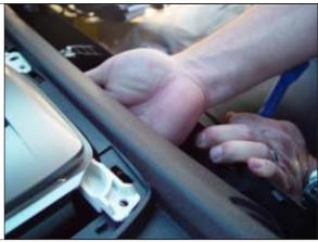
**STEP 10.** Lift the plastic white shifter frame and stock shifter cover out of the center console. Access the LED bulb and wiring and twist the bulb housing to disconnect it from the frame.
