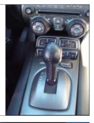
**STEP 2.** Carefully pry out the plastic access panel on the front of the shifter knob.
