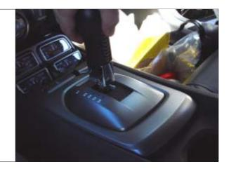
**STEP 5.** Gently pry off the center console trim around the shifter being careful not to scratch the finish.
