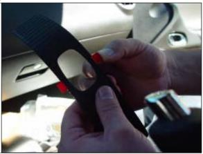
**STEP 13.** With the red indicator firmly in place. Apply a drop of instant adhesive into the back square access hole of the black plastic slider to lock the red indicator in place.
