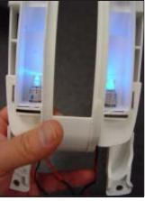
**STEP 19.** Place the black plastic slider into the track of the white plastic frame with the original red indicator on the driver's side of the vehicle (the newly installed indicator on the passenger side). Then snap the Hurst plate onto the white plastic frame making sure the cut-outs on the plate engage the tabs on the white plastic frame on all four (4) ears.
