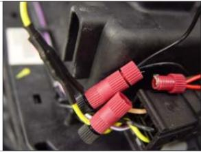
STEP 18. Ensure that all the ABL LEDs' red wires are tapped into the vehicle's yellow wire and all the ABL LEDs' black wires are tapped into the vehicle's black wire before the original LED bulb and resistor pack (NOT between). Test to ensure that the new ABL LEDs illuminate by (recon necting battery if previously disconnected) turning on the vehicles head light or by depressing the brake peddle and turning the ignition ket to the "on" position.
