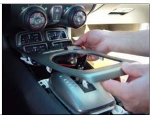
STEP 7. Unscrew the four (4) bolts holding the white plastic shifter cover frame to the center console.
