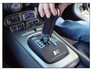
**STEP 25.** Reinstall the plastic access panel on the front of the shifter knob.
