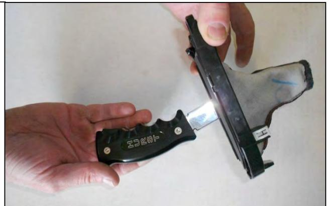
9. Zip tie the shift boot to the pistol grip. There is a groove machined into the handle that is intended for the zip tie to lock into.
