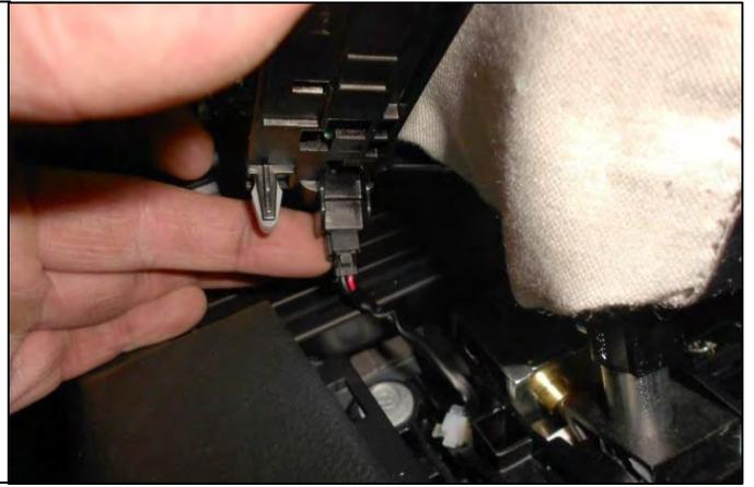
**CAUTION:** With the engine off, the emergency brake set and the front and rear wheels blocked, move the shift handle back far enough to gain access to the two Phillips screws that bolt the shift handle to the lower stick.
