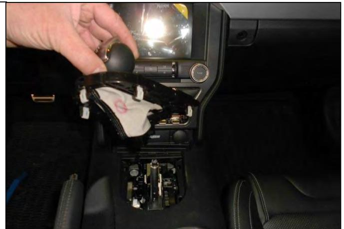
5. Release the locking tabs that secure the shift boot and gear select indicator to the shift handle.
