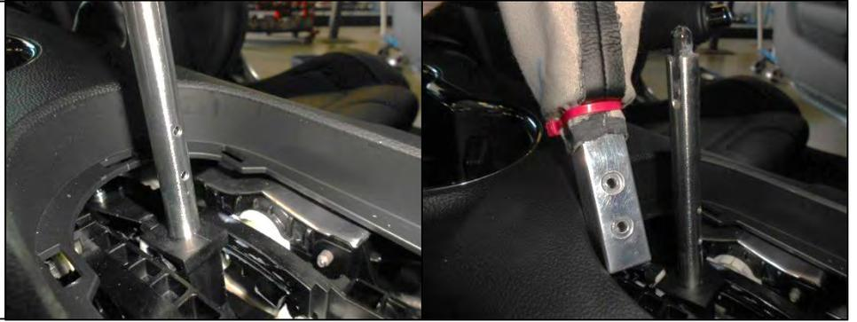
11. With the shift boot still inverted slide the Hurst pistol grip down over the lower stick and secure it in place using the two provided set screws.
