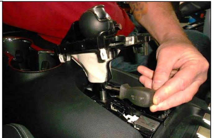
4. Remove the two Phillips screws then pull up on the shift handle to remove it.
