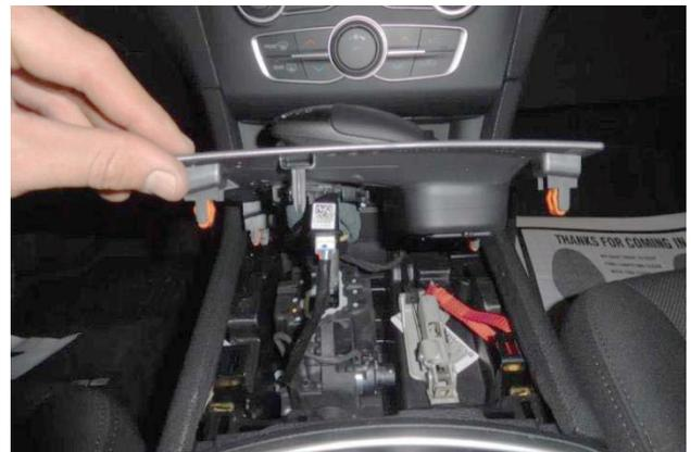
4. Lift up on bezel then unplug shift handle harness connector.
