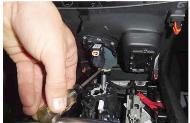
5. Remove factory set screw located at base of shift handle. Pull straight up on shift handle to remove handle and bezel assembly.
