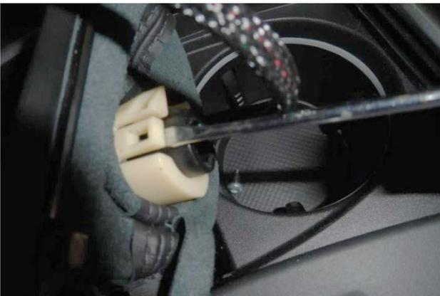
8. Release clips (x2) that mount shift boot retaining collar to shift handle.
