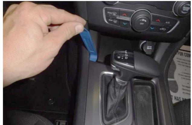
3. Pry up front corners on console bezel then work your way around it to release remaining clips.
