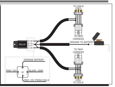
**Figure 2 Optimal High Voltage Supply Harness**
