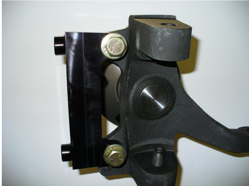
Radial mount bracket installed to inboard side of spindle
