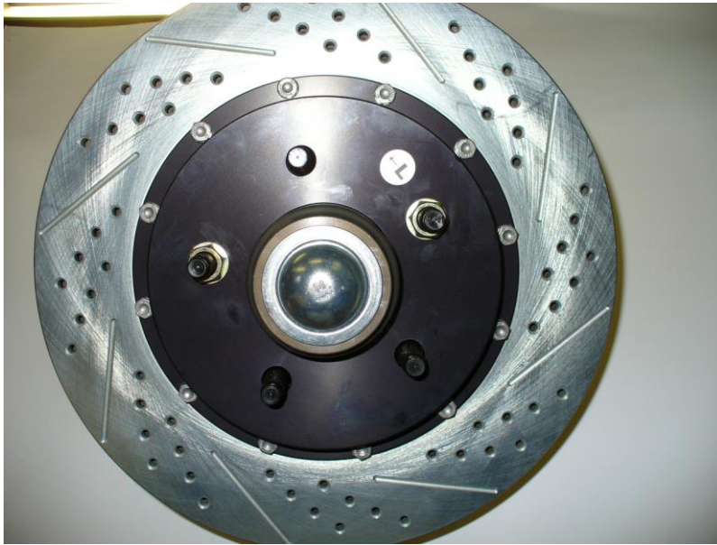
Rotor installed with washers and nuts to prevent marking the hat.
