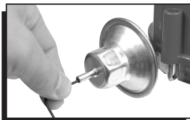
Figure 2 Adjusting the Vacuum Advance.
