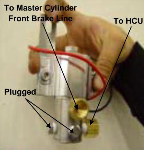
4. Ensure that the new brake line routing is understood prior to installation. However, DO NOT attach lines to solenoid at this time.
