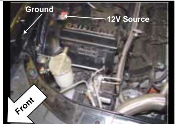
10. Switch wiring can be run through the firewall by going through the grommet for the hood latch release cable.
