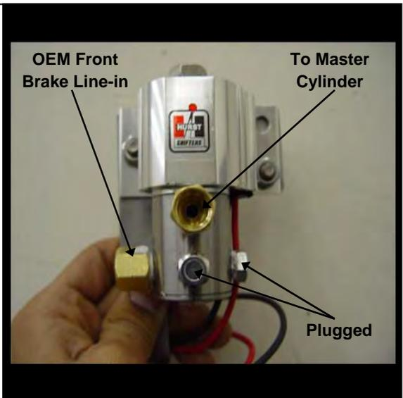
4. Ensure that the new brake line routing is understood prior to installation. However, DO NOT attach lines to solenoid at this time.
