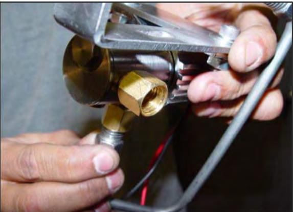
7. Install Hurst Roll Control system and bracket assembly.
