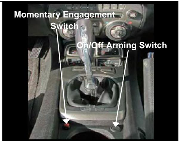
12. Reconnect battery and turn ignition switch to the "ON" position. While still in park and NOT depressing your brake pedal, activate and engage your Hurst Roll/Control system (make sure you can hear the clicking of the solenoid) several times and check fuse. If fuse is burned, check all electrical connections for a short and correct any problems immediately.
