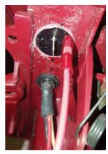
17. Install **terminal (11)** on momentary switch red wire then plug it into On/Off switch.
