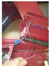
Install terminal (11) to red wire (6) then plug it into on/off switch reaming post. Install fuse holder (10).
