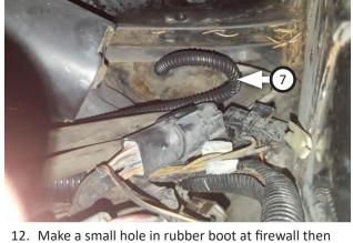
Make a small hole in rubber boot at firewall ther draw power wire through it to inside of vehicle. Cover power wire with split sleeve (7).
