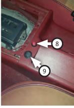
14. Drill and mount **On/Off switch (9)** and **lit momentary switch (8)** to center console as shown.
