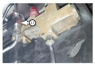
Install provided inverted flare plug (17) to lower block where brake line was removed.
