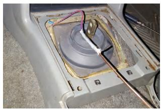
13. To mount switches on center console, pull carpet back then draw power wire through to center console as shown.
