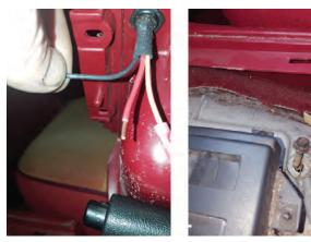
Extend momentary switch black ground wire with splice (13), black wire (5) and eyelet (12). Ground this wire to chassis (this kit was grounded at shifter).
