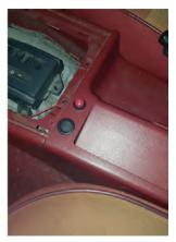
19. Attach red wire to a power source using **tap connector** (15) if necessary.
