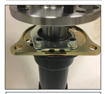
**4**. Next, install the bearing retainer (**not supplied**) and secure it with the factory hardware.
