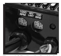
**Figure 3 Adjusting the Rev Limiter.**
