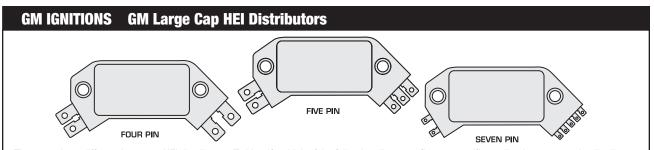
There are three different large cap HEI distributors. To identify which of the following diagrams fit your specific application, remove the distributor cap and rotor and locate the ignition module at the base of the distributor. Count the number of terminals on both ends of the module and follow the corresponding diagram. GM used 4, 5 and 7-pin modules in these distributors.
