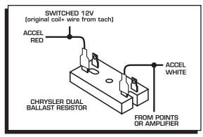
**Figure 4 Wiring the Dual Ballast Resistor.**
