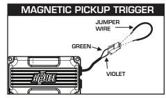
Figure 8 Checking for Spark with Magnetic Pickup.
