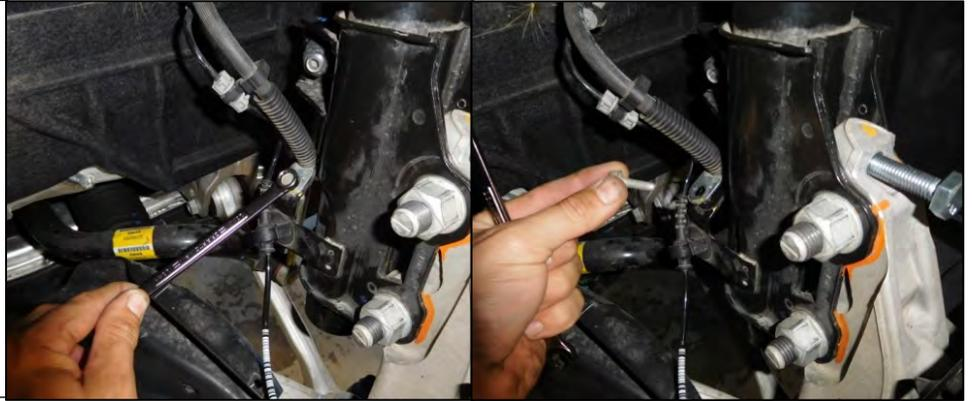
17. Remove the upper sway bar link using a box end wrench with an allen wrench. Once the nut is removed, slide the threaded end of the sway bar link out of the strut assembly.
