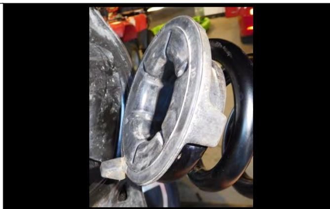
12. The lower spring rubber has a tab that aligns with a slotted hole in the spring pocket of the lower control arm. Install the spring into the lower control arm ensuring that the tab lines up with the hole.
