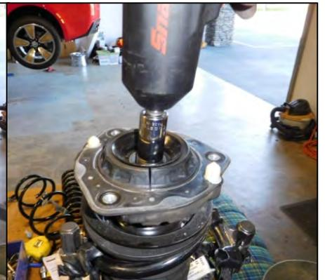
26. Remove the upper cup and rubber boot before removing the spring.
