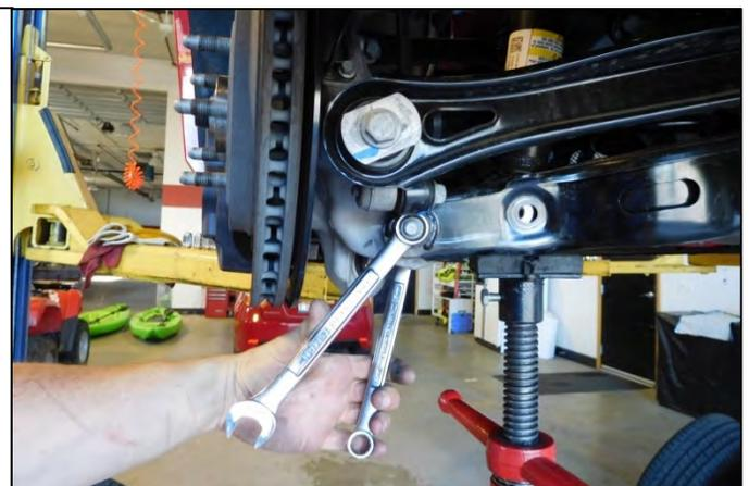
6. Make an alignment mark on the inner rear control arm washer and control arm.
