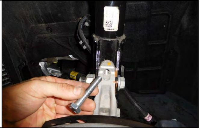
16. Remove the bracket bolt for the rubber brake line. Unclip retainer for the ABS sensor wire. Ensure both are free from the strut and don't have any tension on them.
