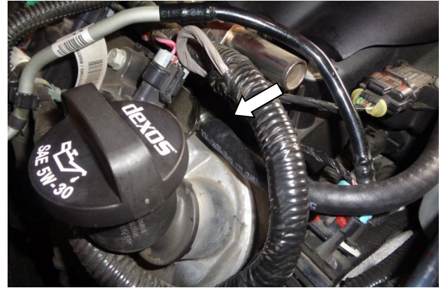
22. Push one end of the 5/16" ID hose (27) onto the metal tube from which the PCV line was disconnected at Step 7.
