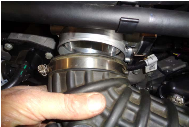
6. Remove the intake tube from the throttle body.
