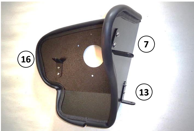
13. Attach brackets to airbox (15) at the locations shown, using ¼" screws (9) (on the bracket side), and flat washers (14), lock washers (4) and nuts (5) (on the airbox side). NOTE: Orient tab on bracket (16) upward.
