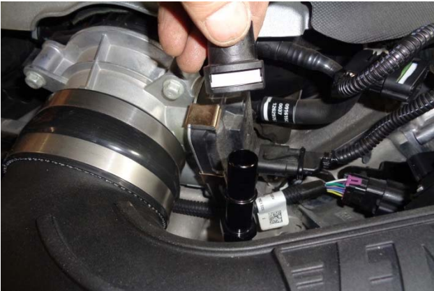
25. Install PCV hose on fitting and check for security.
