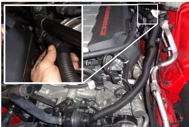
8. Disconnect the back end of the resonator hose.
