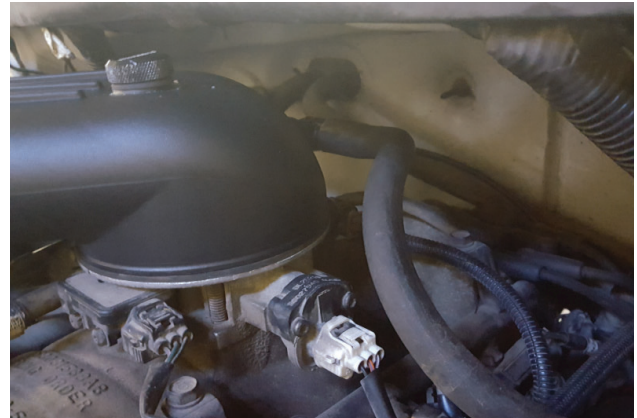
16. Connect breather hose (disconnected step 3) to hose barb on intake tube. If your hose is too short, replace it with fuel hose (10), trimmed to fit. Secure ends using (x2) hose pinch clamps (23).
