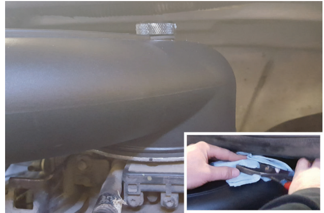
15. Carefully tighten intake knob into tube and throttle body until gasket is slightly compressed.
