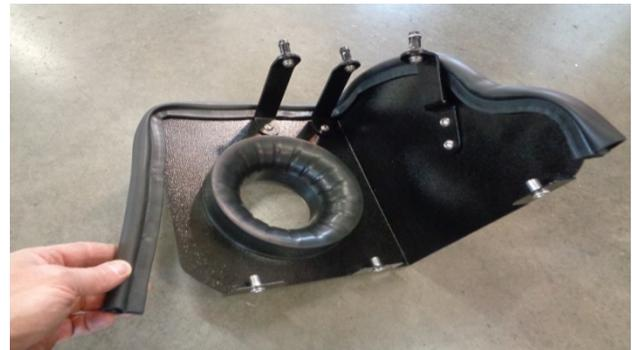
10. Install the rubber trim seal along the outer top and side edges as shown. Press fully into the groove starting from one end. Trim final length with metal shears for proper fitment.
