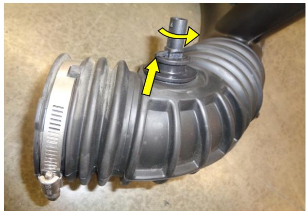
5. Remove the entire stock intake assembly from the vehicle by lifting straight up and out. Turn upside-down on a flat surface and remove the air temp sensor from the intake tube by prying up the locking tab with a flat screwdriver and rotating c-clockwise.
