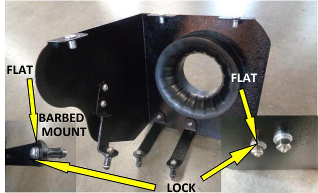
9. Install the metal brackets included in the kit using the supplied 1/4" screws/washers/nuts as shown. Then, install the barbed mounts onto the metal brackets using the 6mm screws/washers.
