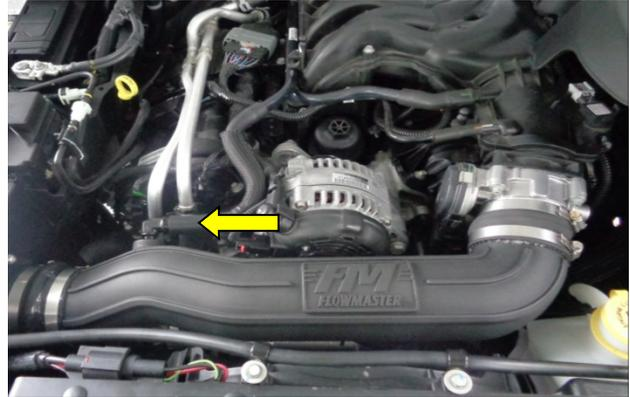
15. Install the FM intake tube assembly onto the air-box and the throttle body\*. Align and tighten all clamps for a satisfactory fit. Slip the crankcase vent hose onto the barbed fitting
