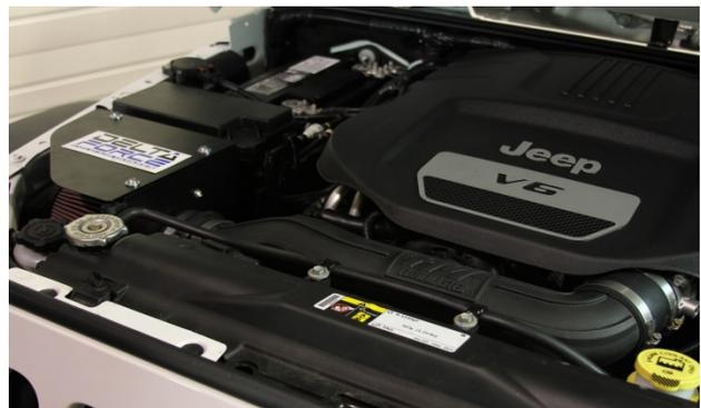
17. Secure the provided cone filter using the included hose clamp in the desired position. If desired, install pre-filter over the cone element. This will help extend the life of the filter by keeping out the larger particles. Using the last three 1/4" screws/washers, secure the air-box lid, re-install the engine cover and the battery cable.
