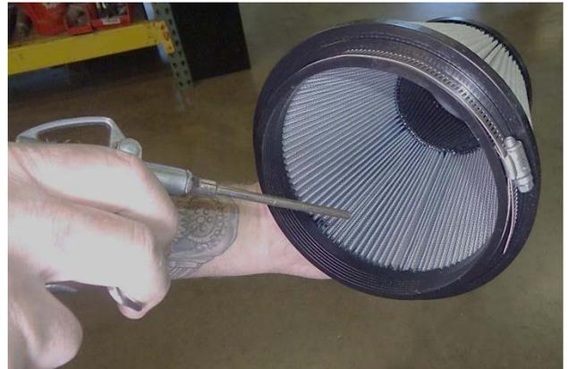
3. **Blow through** the filter, from the inside out. Keep the nozzle moving; do not hold it stationary over one place on the filter.
