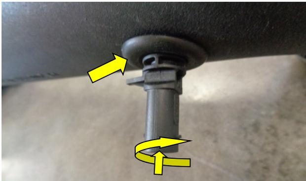
13. Insert the provided rubber grommet
