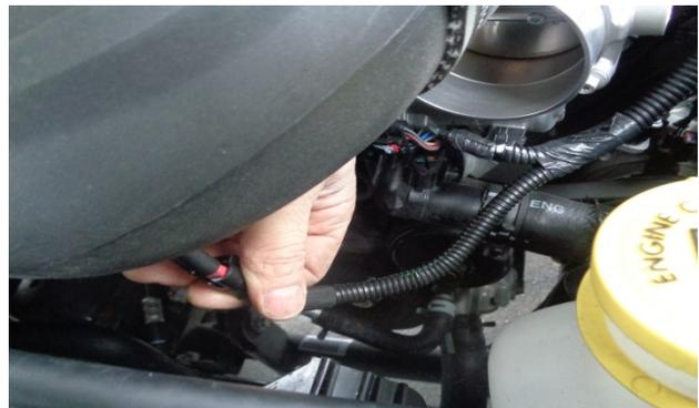
16. \*Due to limited space for access, it may be necessary to attach the air temperature plug during the intake tube attachment process. Make sure that the plug fully engages the retaining tab on the sensor.
